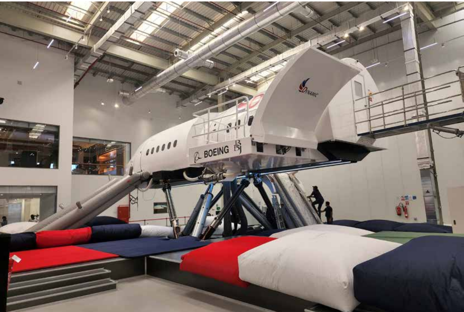
Spatial built this BBJ cabin safety training device for Dynamic Advanced Training. Spatial
