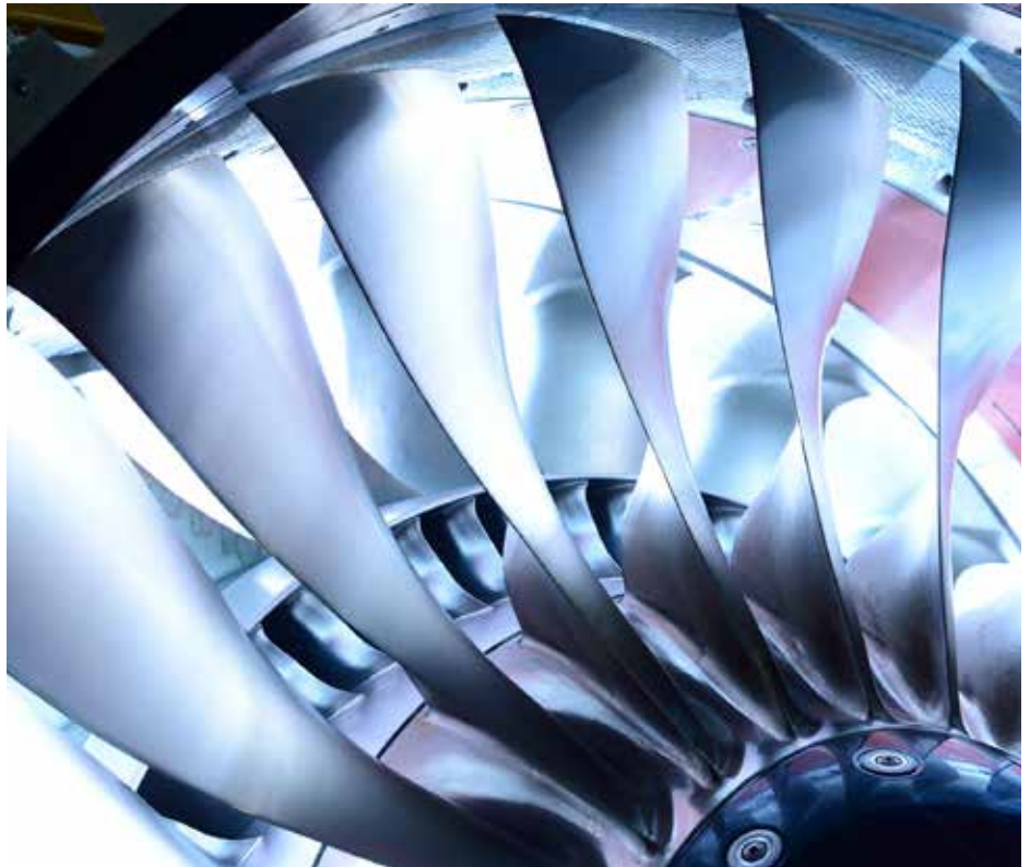
Rolls-Royce introduced a blisked fan on the Pearl 700. Rolls-Royce
