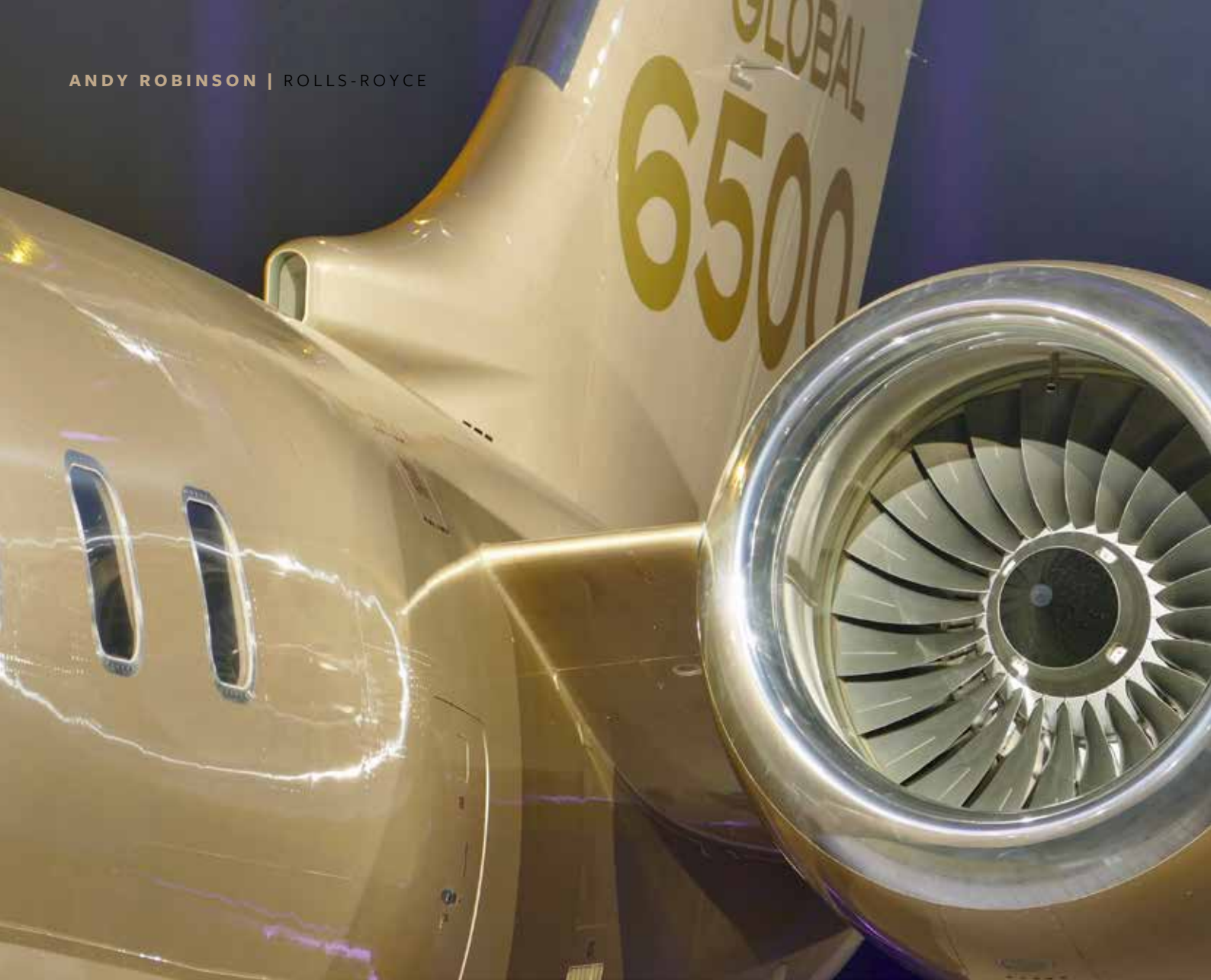
Rolls-Royce developed the Pearl 15 for Bombardier's Global 5500 and 6500
